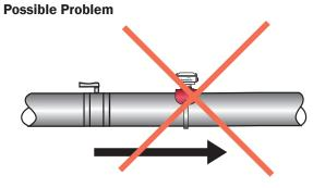
Post-valve cavitation can create air pocket
