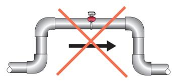
Allows air pockets to form at sensor
