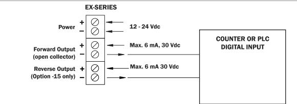
See Dual FT430/440 Diagram for an example of bidirectional connections.
